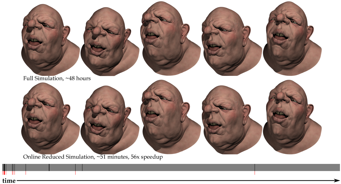
Figure 1: We learn fast subspace models on-the-fly to accelerate deformable simulation: (Top) Ground truth frames from a 1000-frame deformable character simulation with 165,941 tetrahedra and Arruda-Boyce material which took 48 hours (174,521 seconds). (Middle) Frames from our online integrator which were generated in only 51 minutes (3,101 seconds) – 56.28 \times faster – by learning a fast 11-dimensional subspace model on-the-fly (Bottom) Visualization of the temporal behavior of the online integrator reveal full steps (in black), reduced steps (in gray), and basis updates (red ticks). A reduced basis is detected quickly, and the first “skip” occurs at timestep 2. Only a handful of full steps are needed, and our reduced solver computes over 98% of the steps.
